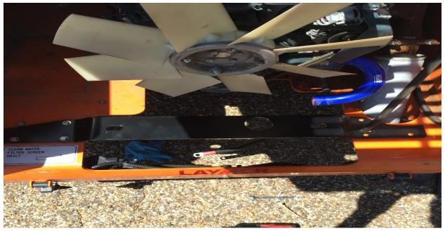
16a. Slide and center the new radiator mount plate all the way to the left hand side. Install 3 existing bolts on the left side securing water pump. This will help with the fan clearance. Drill 3 holes with a ¼" bit on the right hand side. Install right hand side mounting bolts.
