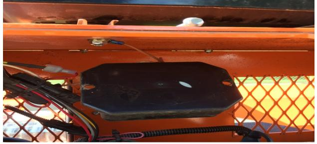
21. Install new top radiator mounting plate (1000041) between the frame and the 3 way shutdown box. Use 2 screws (407502), washers (011321) & nuts (440628) in parts kit. Leave the bolts slightly loose to aid in radiator alignment
