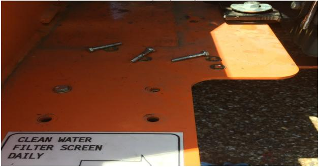
19.Install new bottom radiator mount (1000040) using 3 bolts (441568) & nuts (440636)
