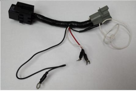
b. 4. Remove loom and tape from jumper. Disconnect relay.
