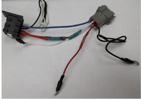
9. Tape the wires together into a bundle and re-loom the jumper.
