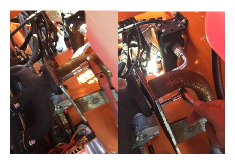
3. Remove existing exhaust manifold downpipe and remove muffler. Discard downpipe.
