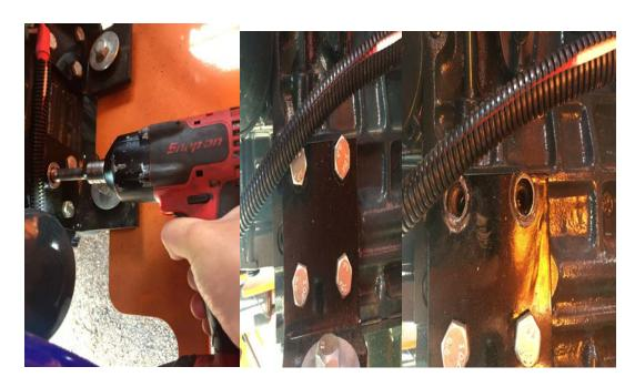
5. Attach muffler support bracket onto the right rear motor mount. Apply thread locker to both bolts and torque to 50 Ft. Lbs. using the 17 MM socket.
