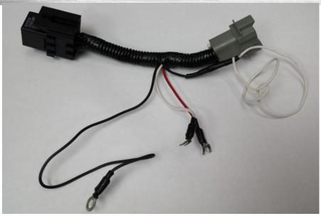
4. Remove loom and tape from jumper. Disconnect relay.
