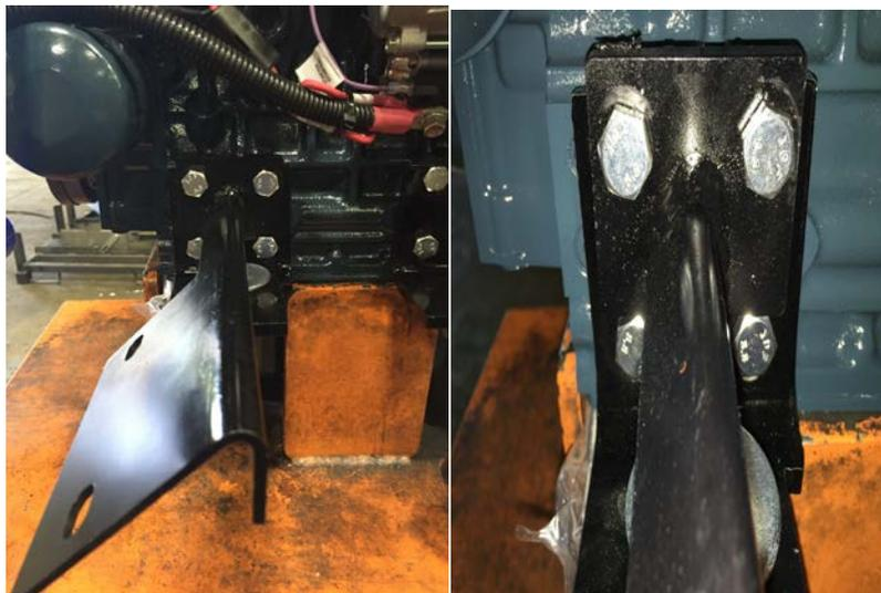
7. Install muffler to down pipe. Install muffler to assembly to new muffler mount bracket.
