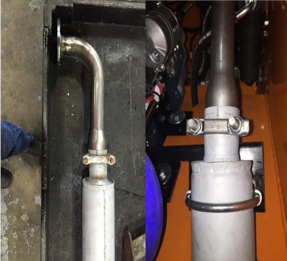
8. Install exhaust muffler U-bolt clamp and leave slightly loose. Install muffler down pipe assembly to exhaust manifold. Torque manifold bolts to ? Tighten the U-bolt clamp to ?
