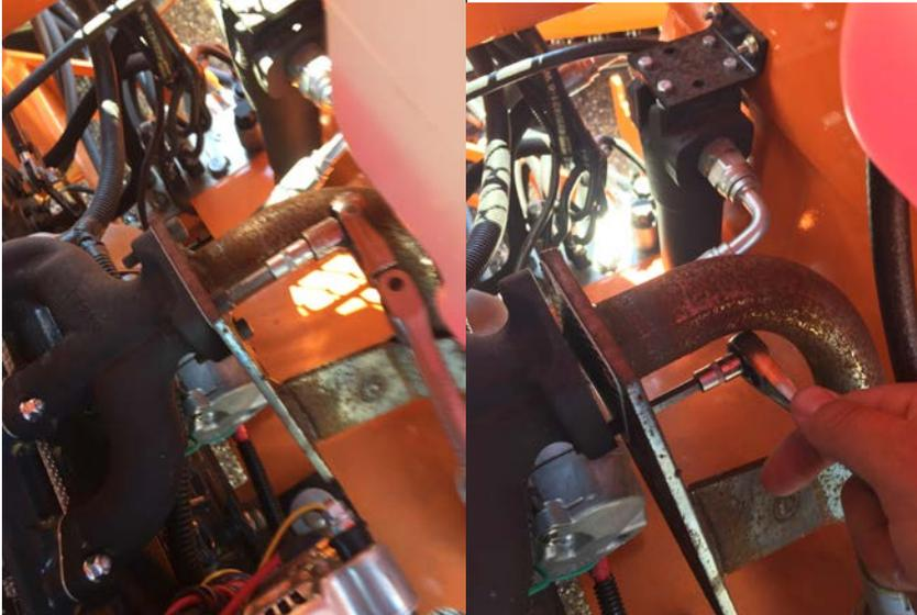
3. Remove existing exhaust manifold downpipe and remove muffler. Discard downpipe.
