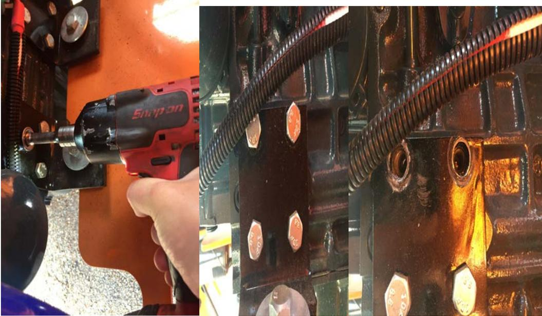
5. Attach muffler support bracket onto the right rear motor mount. Apply thread locker to both bolts and torque to 50 Ft. Lbs. using the 17 MM socket.
