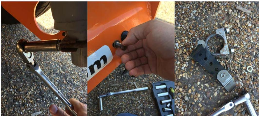
2. Next remove the exhaust down pipe bolts (4 ea.)
